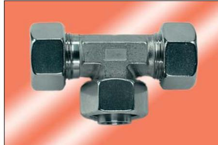
Port D1 is pre-assembled. Final assembly in appropriate body with approx. 1/2 turn beyond the point of clearly perceptible resistance.
