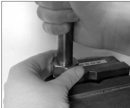
4. Check whether a visible collar has formed on the pipe in front of the (first) cutting edge.
