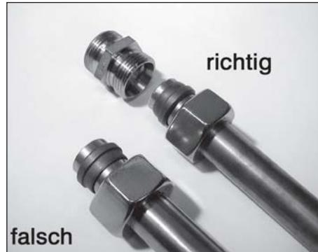
3. Screw the union nut onto the pre-assembly connection piece as far as possible by hand. At the same time, press the pipe against the stop. As soon as the cutting ring has cut into the pipe, the tightening moment will increase noticeably. A flag at the union nut facilitates the observation of the necessary revolutions. Tighten union nut using a wrench by approx. 1 1/4 revolution. Important: Do not turn the pipe with the nut!
