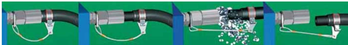
Parker's Hose Whip Restraint System is designed to prevent whipping of a pressurized hose in the event of the hose separating from its fitting. The Hose Whip Restraint System provides an additional level of safety and helps prevent damage to nearby equipment or injury to operators near the failed hose by limiting the whip or travel of the pressurized hose after it breaks free from its hose fitting. Serious damage or injury can occur from whipping hoses, especially at higher pressures.
