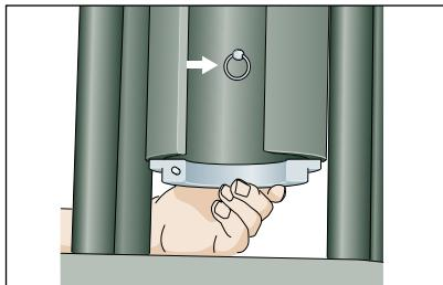
With the pusher in the full up position, lift the back half of the split die ring. Lock it in the up position by pushing the slide pin in (the slide pin is located inside the pusher at the back).
