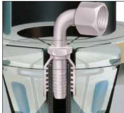
3. (a) Position the fitting on the die step.
